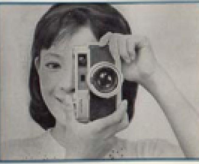
It is best to focus with the right eye when using the horizontal position to permit free and rapid use of the film advance lever. The lever contains a double-exposure prevention device; the shutter locks after each picture is taken.
